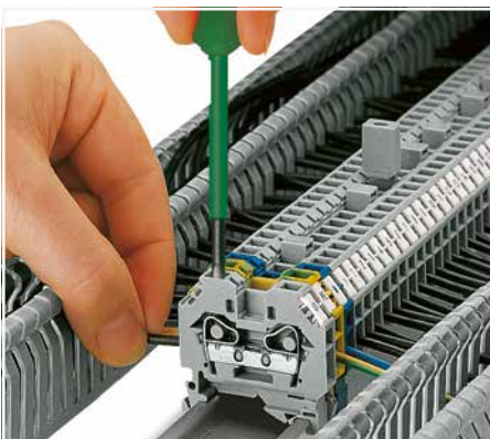
CAGE CLAMP® connection Inserting a conductor. With ferruled conductors, it is necessary to use a terminal block one size larger than the conductor's nominal cross section.
