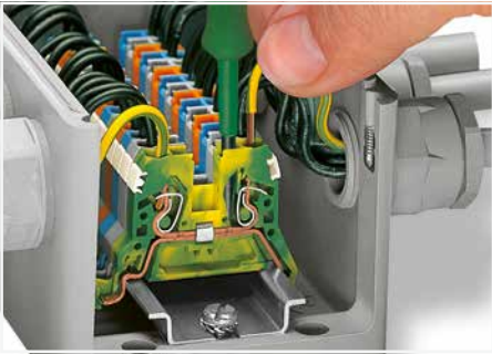
CAGE CLAMP® termination: Inserting a conductor via operating tool (0.08 ... 4 mm 2 "f-st"). With ferruled conductors, it is necessary to use a terminal block one size smaller than the conductor's nominal cross section.
