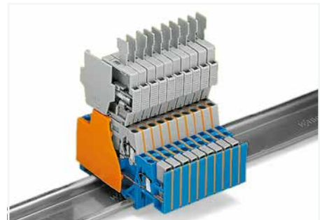
When double-deck terminal blocks are used with a fuse plug (6 mm wide) in the receptacle (top) level, the extra width can be compensated for the 280 Series (5 mm wide) via an intermediate plate (1.1 mm thick). If required, this special intermediate plate still allows commoning on the lower level via push-in adjacent jumpers (280-402).
