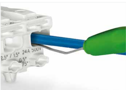
Conductor removal: Slide disconnection tool beneath the conductor and pull both conductor and tool out.
