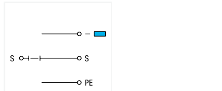
Actuator disconnect terminal block; with ground connection; for phase interruption
