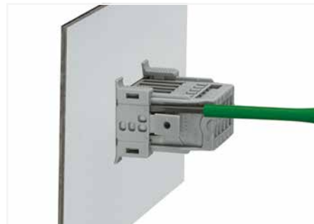
For removal, insert operating tool (2.5 mm blade) into release slot.
