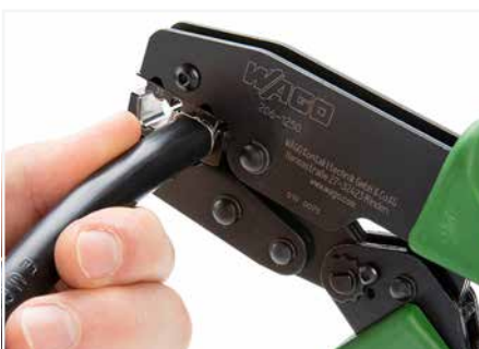
Squeeze handles until ratchet mechanism is released.
