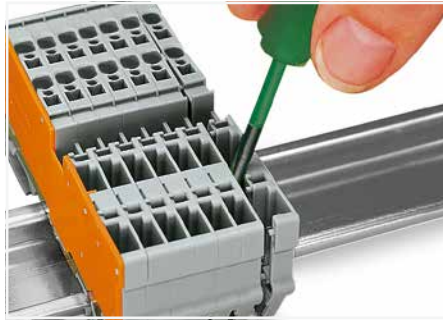
Open the assembly by laterally sliding a block via operating tool and remove terminal block via release lever.
