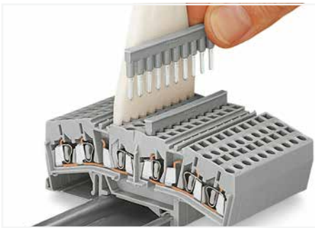
Multiplying potentials via 10-way comb-style jumper bar. (only possible in the terminal block's center)
