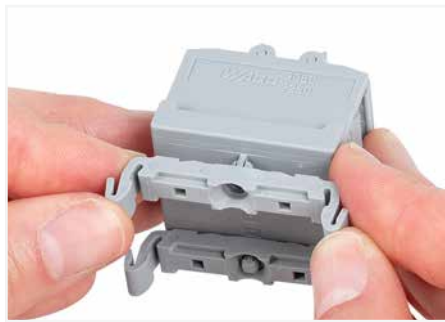
Terminal strip; with snap-in mounting feet Snapping a mounting foot (209-120) (Distance between mounting feet: approx. 20 ... 25 mm)
