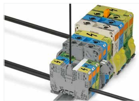
Always push voltage tap (283-407) down into the terminal block until fully inserted!
