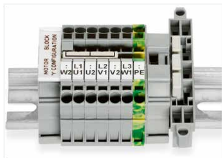
This star point jumper has been specially developed to create a "star point" and is used on motor terminal boards equipped with rail-mount terminal blocks TOPJOB® S.
