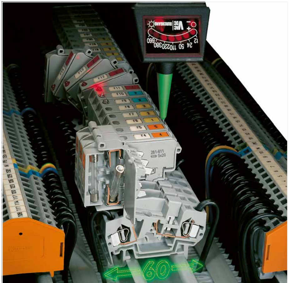
CAGE CLAMP® connection Inserting a conductor. With ferruled conductors, it is necessary to use a terminal block one size smaller than the conductor's nominal cross section.
