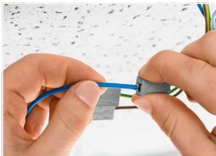
To connect: Press button fully, insert stripped conductor into square entry and release.
