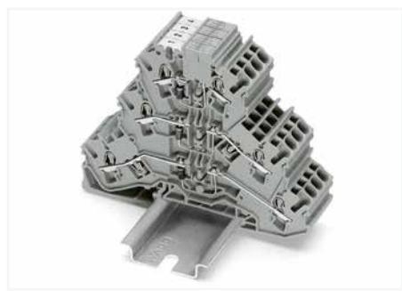
Triple-deck diode terminal blocks were specifically devel- oped for custom diode circuits, such as lamp test and col- lective fault signal circuits. These terminal blocks provide high-density wiring in a width of just 5.2 mm. Push-in type jumper bars provide additional options for custom circuit design.
