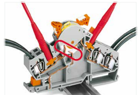
Disconnect link in notched position "I" (terminal block 2) Disconnect link in notched position "TEST" (terminal block 1) – measurement testing Before moving the disconnect link of terminal block 1 into the notched "TEST" position, the reference current meter must be inserted into the test socket of terminal block 1.
