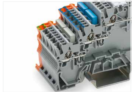
Ground commoning: For sensor and actuator terminal blocks without ground connection to the DIN-rail, the ground connection can be performed by commoning to the terminal block with a ground foot.
