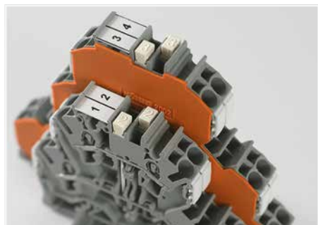
Created for double- and triple-deck terminal blocks TOPJOB® S, the vertical jumpers can common two or three levels. Clearly marked numerals ("2" and "3") distinguish the double-deck (2002-492) and triple-deck vertical jumpers (2002-493), even when inserted.
