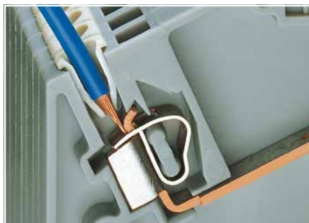
Insulation stop: Prevents the conductor insulation from being pushed into the clamping unit. (Available for terminal blocks up to 4 mm 2 /12 AWG)
