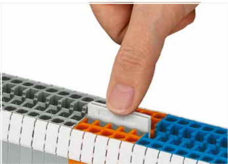
Push jumper bars down firmly until fully inserted. When using multipole bars, push alternately on the right and then left side until installed. Push-in type jumper bars 1-3-5-7 or 1-4-7 are available upon request.
