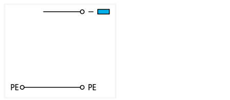
Actuator supply terminal block; with ground connection; power supply from control panel side; with end plate
