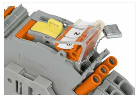
A lock-out seal can be used on the disconnect link in operating position I in combination with an end and separator plate (2007-8893 or 2007-8894).
