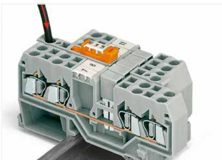
Power distribution using disconnect link in supply line – disconnection of all outputs.
