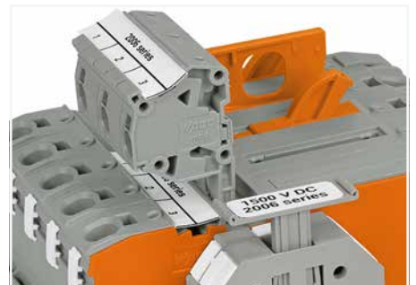
Alternatively, measurement can also be performed using Connectors (2006-511) from terminal block 1 to 2. Spacer modules (2006-549) must be used to compensate for the 15 mm terminal block width.
