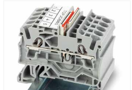
Locate red stripes of the staggered jumpers on the inside. Insert staggered jumper and push down until it hits back-stop.
