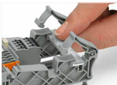
Place the busbar in the carrier holder.
