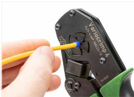
Squeeze handles until ratchet mechanism is released.
