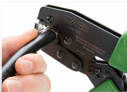
Squeeze handles until ratchet mechanism is released.
