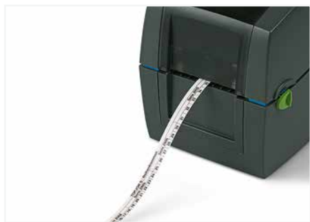
Printing a marking strip (2009-110) via Smart Printer.
