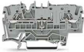
2-conductor carrier terminal block; for 35 x 15 mm and 35 x 7.5 mm DIN-rails; 2.5 mm 2 ; Push-in CAGE CLAMP®
