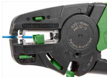
Partially stripping a conductor.
