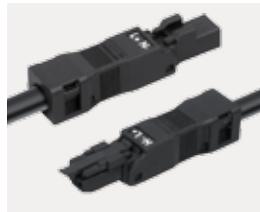
WINSTA® MINI/MINI special 0.25 ... 1.5 mm 2 / 16 A / 400 V
