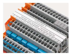
TOPJOB® S Sensor/Actuator Terminal Blocks can be marked in multiple ways. Marking strips (2009-110) offer the fastest and easiest possibility. Multi-line marking simplifies the labeling of a terminal block's function, allowing individual signals and groups to be simultaneously marked.
