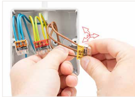
Removal: Hold solid conductor to be removed and twist alternately left and right while pulling the connector.
