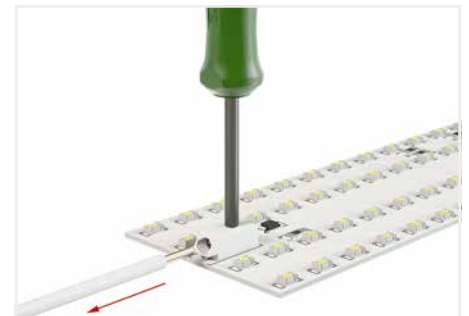
Easy conductor removal (e.g., via 206-859 Operating Tool)
