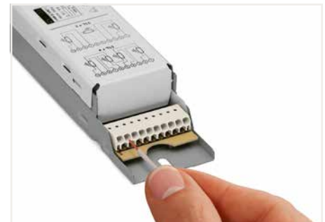
Inserting a conductor via push-in termination.
