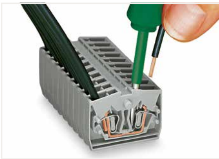
CAGE CLAMP® termination: Inserting a conductor. With ferruled conductors, it is necessary to use a Terminal Block one size smaller than the conductor's nominal cross section.
