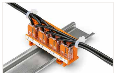
Strain relief via cable ties on the mounting carrier (transverse to the connectors' wiring direction) – clamping units labeled via marking strips (210-334)
