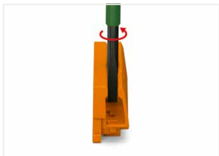
To adjust the mounting carrier, unlock the latch via operating tool (5.5 mm blade) and move the clamping slide to the required width by rotating the tool.
