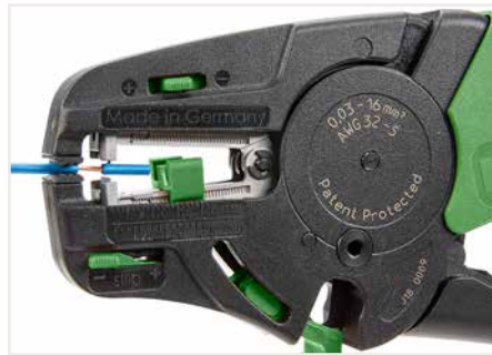
Partially stripping a conductor.
