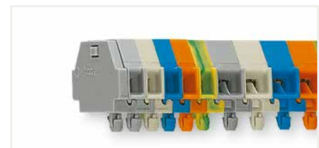
Terminal strip; with snap-in mounting feet; for 0.6 ... 1.2 mm plate thickness; 3.5 mm mounting hole diameter (also for 210-154 Aluminum Rail or with 209-120 Mounting Foot for DIN-35 rail)
