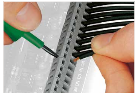
The above-listed operating tools with blade dimensions per DIN 5624 are ideal for operating PCB Terminal Blocks.
