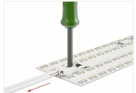
Inserting/removing fine-stranded conductors by lightly pressing on a push-button (e.g. via 206-861 Operating Tool).
