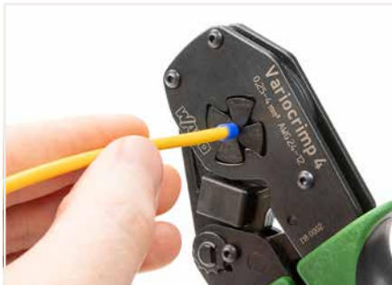
Squeeze handles until ratchet mechanism is released.
