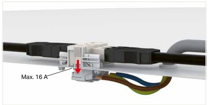
WAGO Linect® Lighting Terminal Blocks are ideal for connecting additional consumers that were not originally planned (e.g., spots). The maximum current between WINSTA® Linect® T-Connector and Lighting Terminal Block is 16 A.
