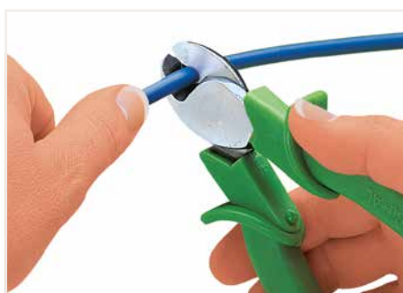
Cutting a cable.
