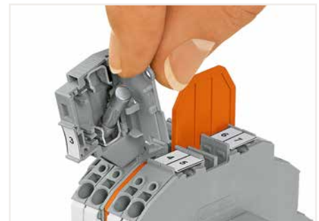
An end plate for fuse disconnect terminal blocks (shown in orange, 2002-1092) is used for additional protection, preventing the fuse holder from being opened. The fuse cannot be replaced until disconnecting the fuse holder from the power supply.
