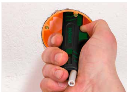
Stripping a cable sheath.
