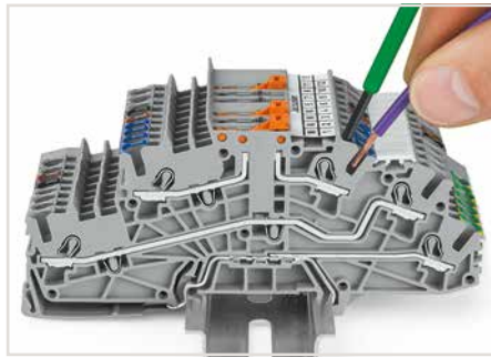
Inserting a conductor via operating tool. Connecting fine-stranded conductors without ferrules, or small cross-sectional conductors that cannot be pushed in, is performed similarly to the original CAGE CLAMP® – just use an operating tool.
