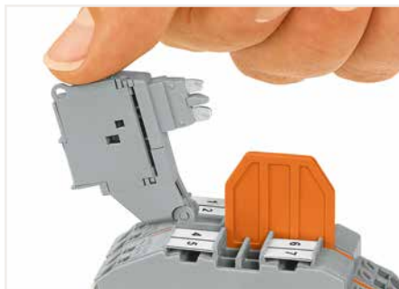
Double-deck fuse disconnect terminal blocks with a pivoting fuse holder (2002-2611, gray) are compatible with disconnect, carrier, through and ground conductor terminal blocks. The fuse holder is also available with a blown fuse LED indicator (e.g., 2002-2611/1000-541 for 12-30 V).
