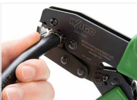
Squeeze handles until ratchet mechanism is released.
