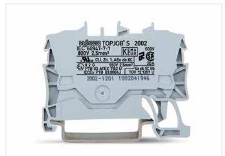
Example of marking (rear): The embossed details on the terminal blocks show the manufacturer's name, the series no., the type of protection Ex e II, the approval no., the approval data and the name of the testing authority.
