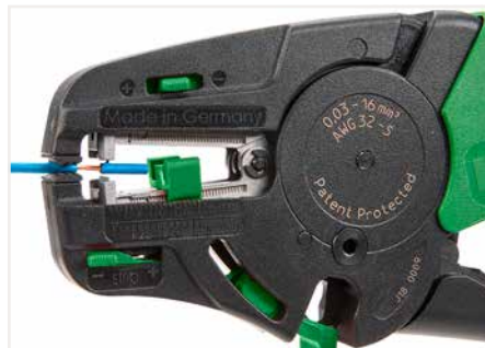
Partially stripping a conductor.
