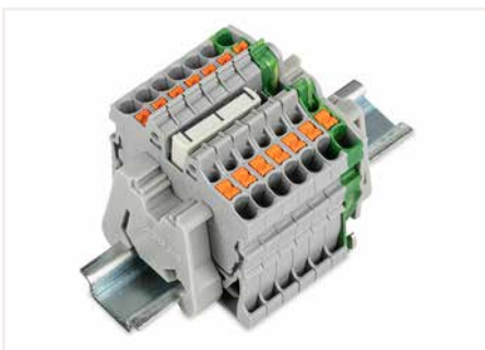
Insert a push-in type jumper bar and push down until it hits the backstop (example shows a 2000-405/011-000 Star Point Jumper).
