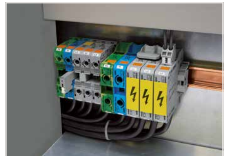
Side-entry wiring means that even larger conductors, which have limited flexibility, can be easily connected.
