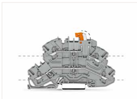
Double-deck disconnect terminal blocks with a pivoting knife disconnect (2002-2671) can be used as through terminal blocks on the lower deck and as disconnect terminal blocks on the upper deck. Besides disconnection and measurement, double-deck carrier terminal blocks (2002-2667) also provide ground conductor functionality.
