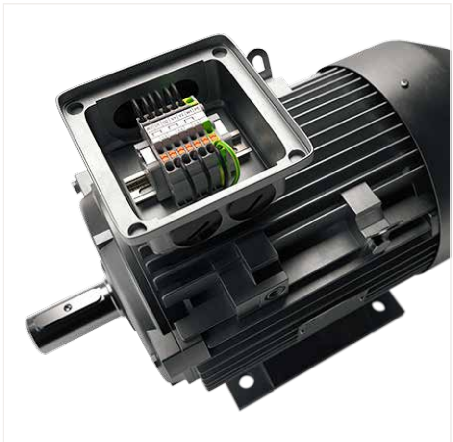
Insert a push-in type jumper bar and push down until it hits the backstop (example shows a 2000-405/011-000 Star Point Jumper).
