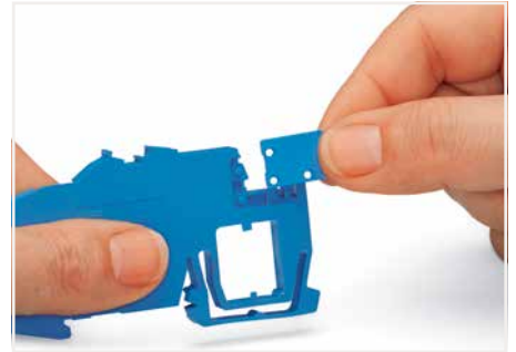
Inserting the separator plate into the busbar carrier to protect the N-busbar against accidental contact.
