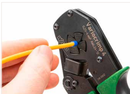
Squeeze handles until ratchet mechanism is released.
